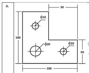
Write NC part program for the machined component of thickness 12 mm to be to drill all the holes as shown in figure. All dimensions are given in mm. Assume speed = 750 RPM and feed = 150 0.2/5/5 mm/min.
