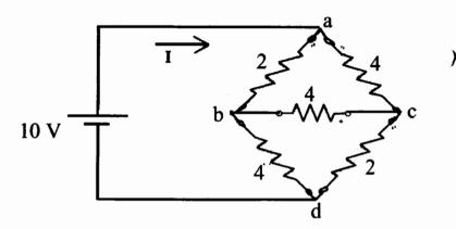
c) Find V and I in the given circuit by using Superposition theorem
